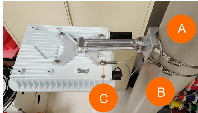
Figure 13: Attaching the security cable
